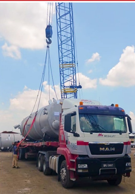
Cargo: Tanks (14 units) Dimension: 15.50 m x W2.80 m x H2.80 m Weight: 12 ton each
