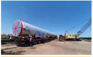
We recently transported two units of Splitting Column known to be the world's largest. Standing at 4.20 m height and over 30 meters long, we loaded them at client's fabrication yard to a private jetty for the RORO onto a barge to be exported.
