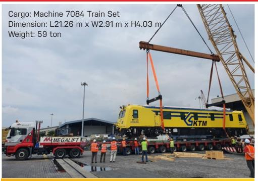
Megalift received the Machine Train Set in Port Klang that was shipped via RORO vessel from Germany. We then transported to Shah Alam and offloaded using two sets of mobile cranes.
