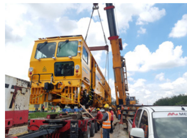
Cargo: Duomatic Machine Dimension: L18.54 m x W2.76 m x H3.75 m Weight: 61 ton each
